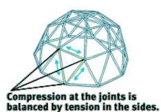
opposite side (see <u>Straw Shape</u>). The geodesic dome's design distributes loads over all of the different triangles that comprise it.
