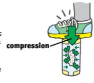
a person's weight. The load is distributed evenly by the material inside the tube. The sand's tendency to spread out is resisted by the sides of the tube, which hold it in and enable it to support the load. In construction, a thin-walled column can be filled with inexpensive material which still greatly increases the column's strength in compression.
