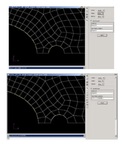
Mesh after Modify->Node -> Move (a single node on the left side of the circular hole moved closer to the location of maximum stress).
