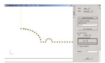
Curve Based mesh seed for 4mm mesh. Element Constraints: Min Length = 3mm Max Length = 4.8 mm
