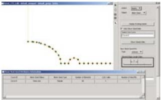
Uniform Element Length mesh seed. Element Length = 4mm.
