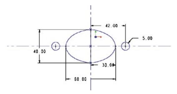
Since the plate is symmetrical in both the x and y directions, a quarter of the plate is modeled using 2D finite element analysis with a plate thickness of 5mm.
