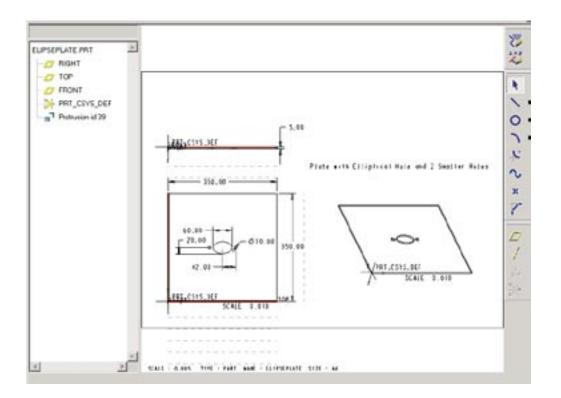
Based on a student number that ends with 1, the distance required for modeling between the center of the ellipse and the center of the smaller circular hole is  $40 + 2^{*}(\text{last digit}) = 42\text{mm}$ .
