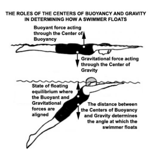
The center of buoyancy relates to the body's volume while the center of gravity relates to the body's mass. Since these two factors normally are different, they are usually sited in different areas of the body. The distance between the centers of gravity and buoyancy usually is greater for males than females.
