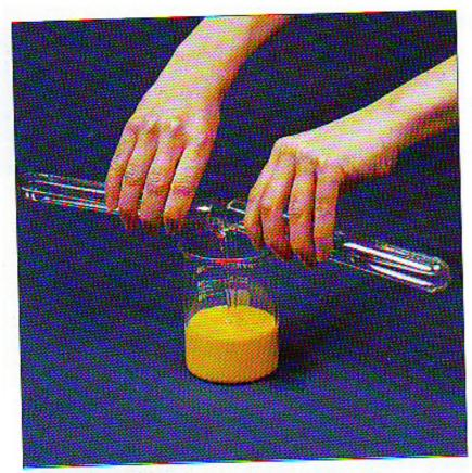
potassium iodide and lead nitrate is a spectacular example of a double replacement reaction.
