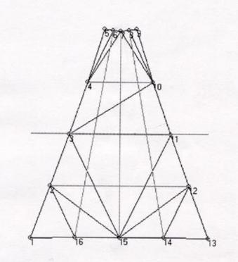
Pattern 2000 (Birdair) calculates lengths of geodesic curves and flattens triangles.
