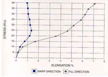
•Modulus of Elasticity (E) E=stress/strain (stress=force/area,strain=dL/L)
