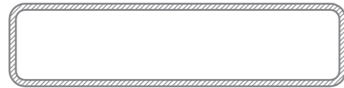
UA6506 65mm x 16mm x 1.2mm Rectangular Hollow
