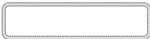
UA6507 65mm x 16mm x 1.4mm Rectangular Hollow
