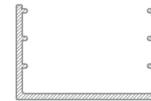
UA2096 38.10mm x 25.40mm Handrail Channel
