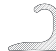
UA1413 24mm x 22mm Heavy Bus Drip Mould
