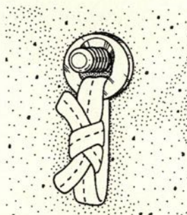
A simple solution for using mangled rivets.
