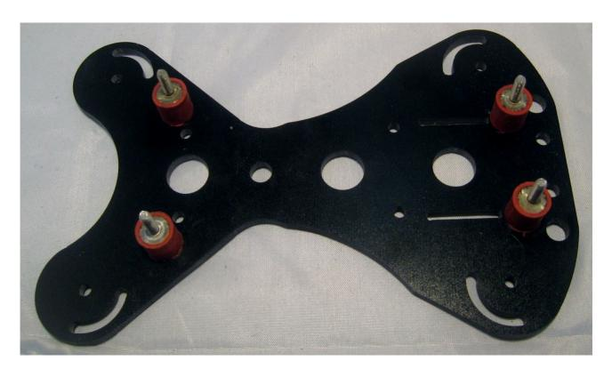
**Step 2**Using the 10mm M3 bolts and M3 lock nuts. Attach the arms as shown bellow.
