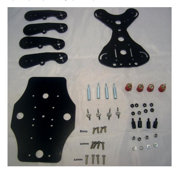
**Step 1**Use the 8mm M3 bolts to bolt in the vibration dampeners like shown in the picture bellow:
