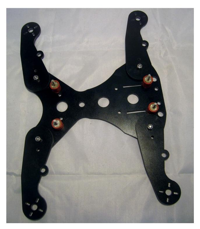
**Step 3**Next, slide the spring washers over the 12mm M3 bolts, insert them into the arms then add the wing nut to the top.
