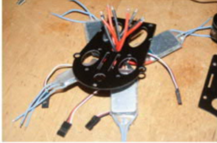
Insert ESC power wires through centre hole
