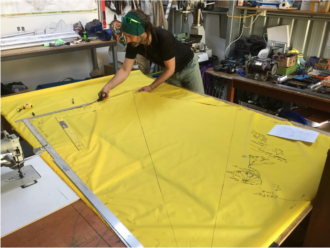
Step 9: Create a "Skirt" from long strips of fabric about 20cm wide. The pattern cut out above will fit the ledge from top to corners. The skirt will be sewn along the bottom edge of the fly to allow the fly to drape over the frame of the sit. The skirt needs to be as long as the circumference of the frame ( $\text{length} \times 2 + \text{width} \times 2$ ).
