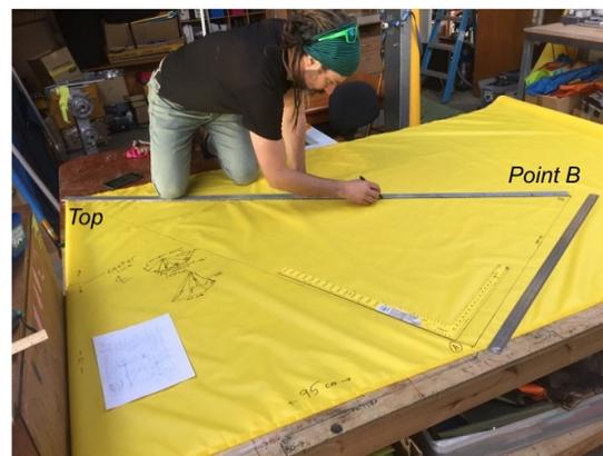
Step 7. Layout Point C. The line from the top to point C is the center “airside”, and the two layers will be sewn together here to create the wrap around fly. The line from the top to Point C makes a right angle to Point B (as the triangle Top-B-C is half of the airside of the fly). **DRAW A LINE FROM TOP TO POINT C.**
