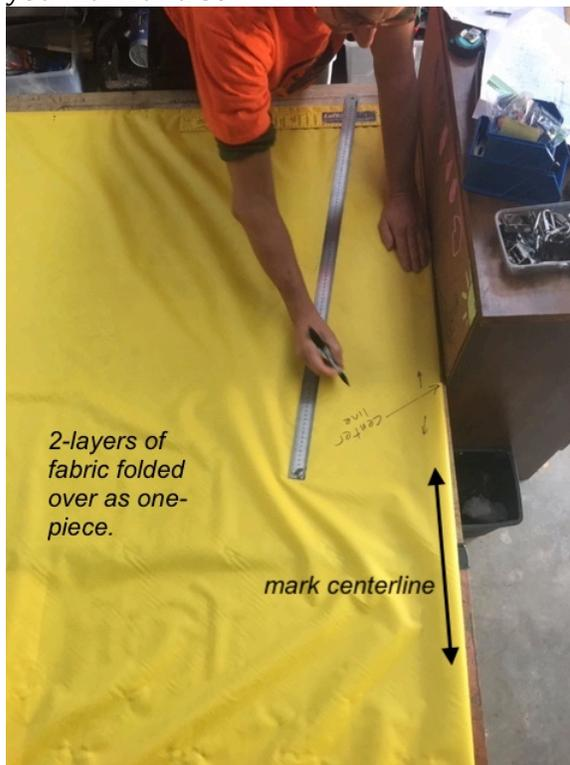
Step 5. Lay out Point A. Measure away from centerline  $\frac{1}{2}$  the length of the sit. Add 3cm depending on how tight you want the fly to fit. For example, if the sit is 190 x 100 cm, measure  $190/2 = 95$ cm (tight fit) out from centerline to mark Point A, the wall side corner. DRAW A LINE FROM THE TOP TO POINT A.
