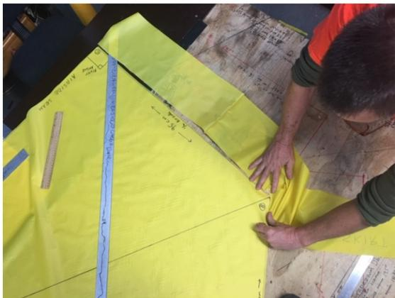
Step 10. Sew the skirt on the bottom (From Point C to B to A and also on other half).
