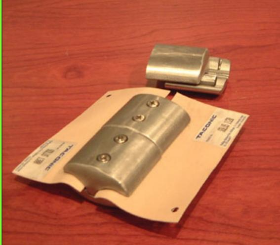
Aluminum Parts with clamped Fibreglass fabric
