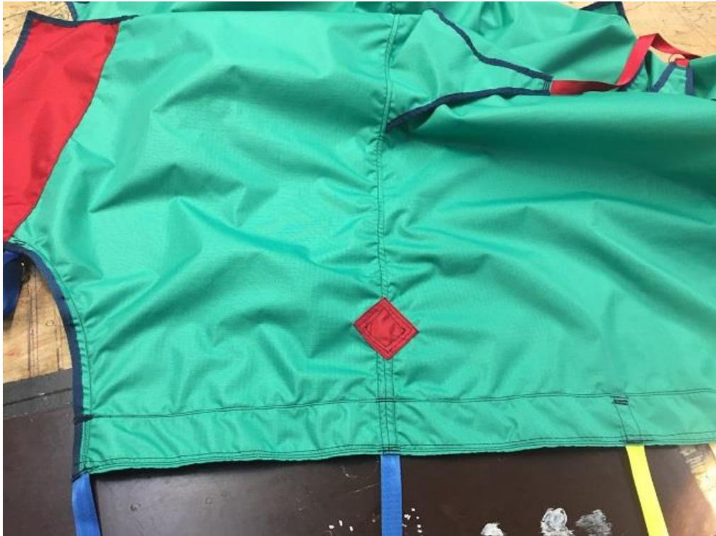
Sew on roller cambuckles, using 3" long pieces of webbing. Two go onto the square patches, the other two on top of the wallside side tensioner webbing 7.5" from wallside. Bartack each.
