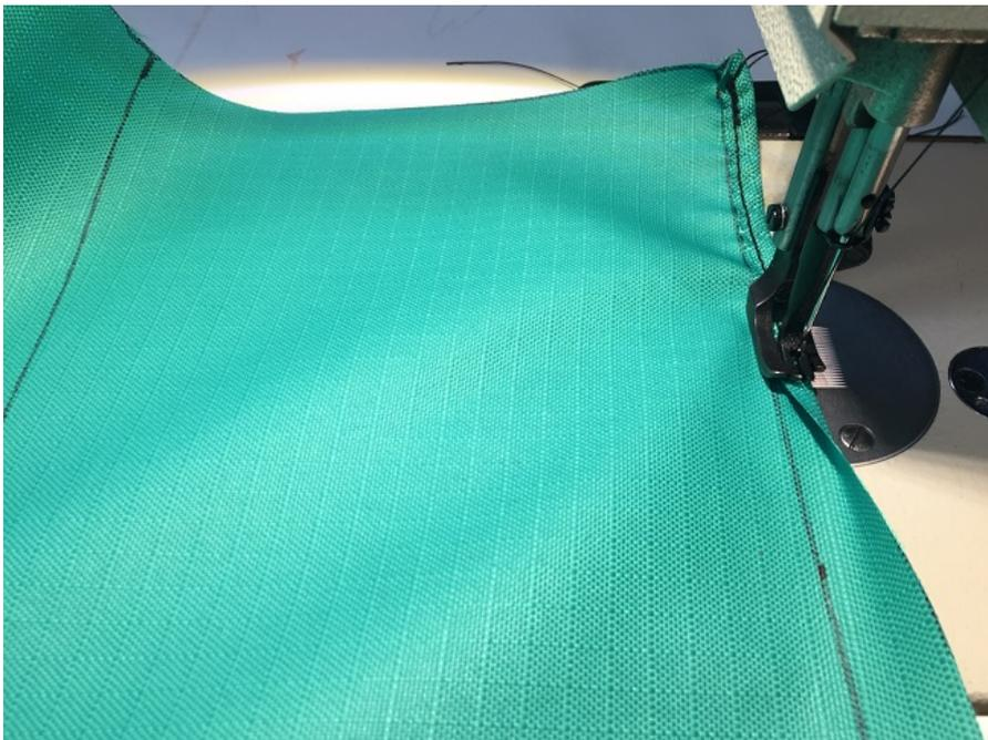
Sew sleeve pieces onto right side of wallside sleeves. Fold over inner edges.
