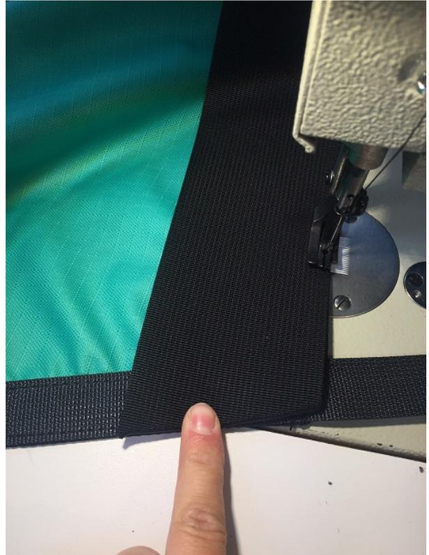
Fold 7" straps into loops and sew onto right side just below sleeves. Bartack 3 x.
