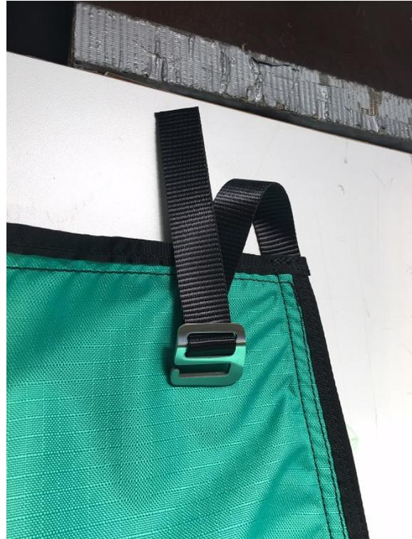
Sew 9½" of the 24" middle strap onto the centre line on wrong side. Bartack 3 x at the end. Do not fold over the end.
