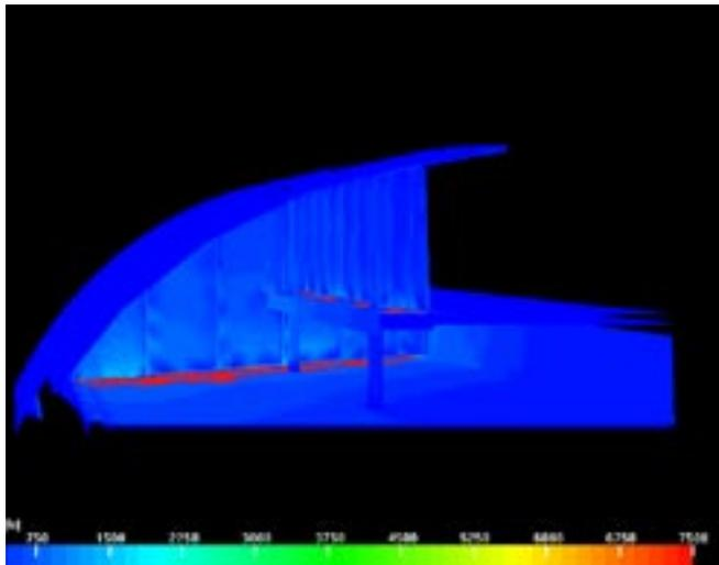
*Left and Below: Lightscape analysis of CAD models allow for rapid experimental design variations to optimize a myriad of light, energy, and aesthetic factor. (John Middendorf GSD project: energy simulation of a Richard Rogers building).*
