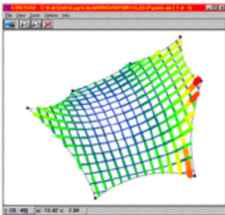
Above and right: EASY tension fabric membrane analysis and design software (\$26000 from Technet)
