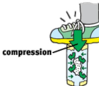
Placing tape over the ends of the tube and filling the tube with sand or salt increases its strength enough to hold a person's weight. The load is distributed evenly by the material inside the tube. The sand's tendency to spread out is resisted by the sides of the tube, which hold it in and enable it to support the load. In construction, a thin-walled column can be filled with inexpensive material which still greatly increases the column's strength in compression.
