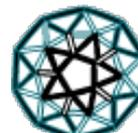
9. Finally, add the last five shorts so that they meet at a single point in the center of the dome. (You might need to stand inside the dome to tape them together.) To test your dome's strength, see how many magazines you can load on top.
