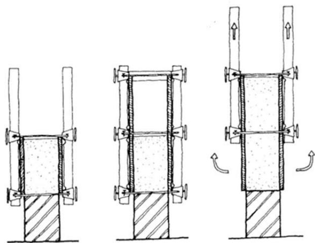
Above: Sliding Formwork for Rammed Earth
