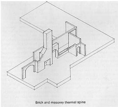
Brick and masonry thermal spine
