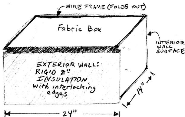
Above: Fabric box with one side of rigid insulation for building segmented earth wall.
