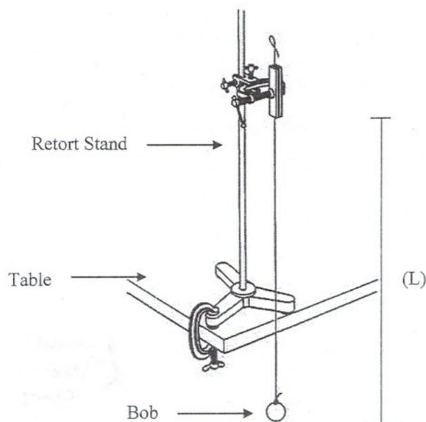
1. Pull the bob about 5cm to one side and then release it. Measure the time ( $t_1$ ) for 10 oscillations and record this in Table 1.
