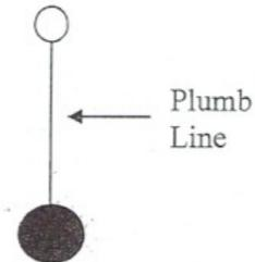
The Centre of Gravity is directly in line with the string.
