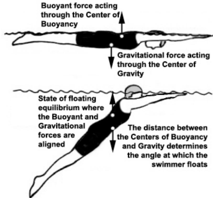
The center of buoyancy relates to the body's volume while the center of gravity relates to the body's mass. Since these two factors normally are different, they are usually sited in different areas of the body. The distance between the centers of gravity and buoyancy usually is greater for males than females.
