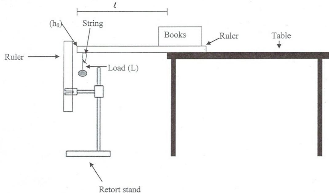
The apparatus is set up as shown in the diagram. Use the back of this sheet to write down your readings and draw a graph.
