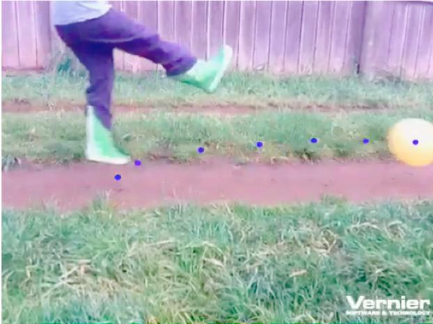
*Taking video and entering points is quick and intuitive. Here, an impulse time of approximately 0.1 seconds can be visualised by watching the video frame by frame and examining the graphs. Distance can also be calibrated.*
