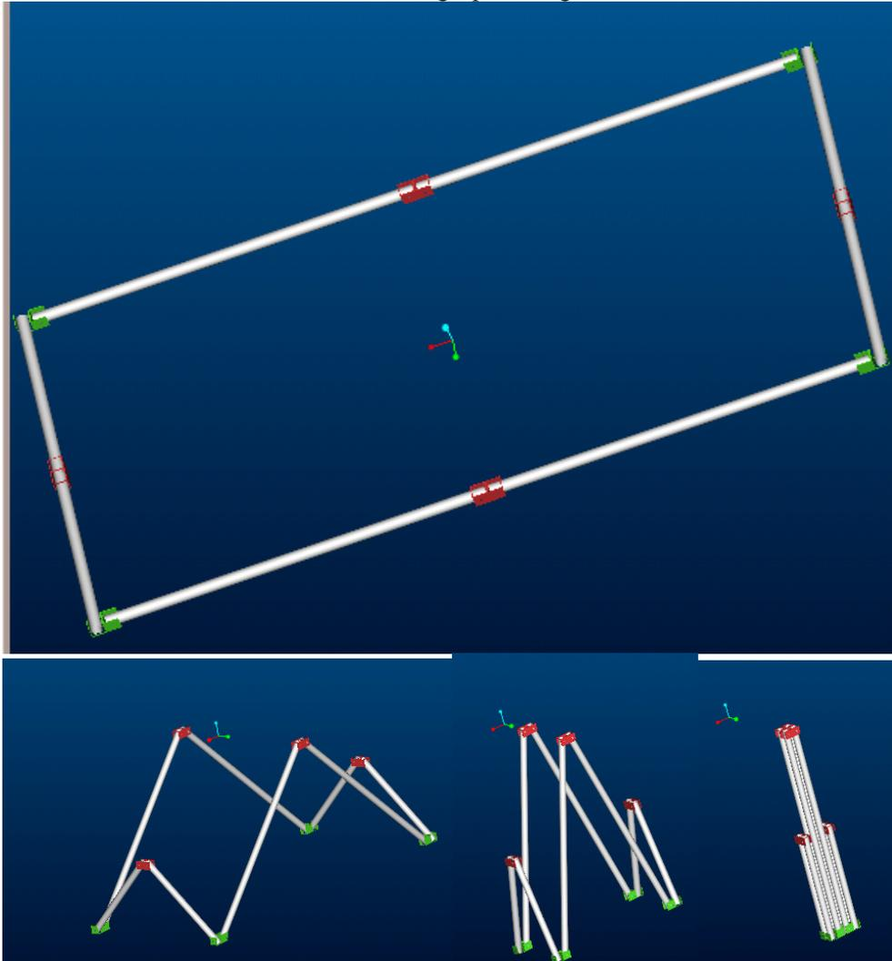
This model used primarily drivers to create the motion and produced predictable results. The main benefit was how it proved the corner and center hinge design was compatible with a closed loop system of tubing.
