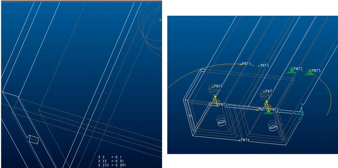
Above Left: using a contact point to measure when the square tubing comes into contact with the hinge. Right: using slots: the idea here was to measure the positions of the points in the slot and have forces applied to stop further travel of the tubing when it came into contact with the hinge. Unfortunately, although I could get these systems to run in simple models, both these methods resulted in major problems when I tried to run them in Mechanica in models that had a total of 18 connections.
