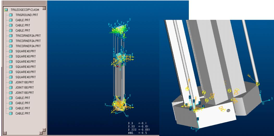
This model uses six 40 inch square tubes, three 180 degree hinge connections, and three 90 degree connectors which angle each tube at 120 degree spacing (the “tri corners”). In addition, the suspension is modelled as cables. Originally, just one cable was used to each tricorner, but I found better results if I added a cable to each tricorner to stabilize the rotation of the tricorners. In the end, I used two for each tricorner, and one had an additional cable to prevent spinning.
