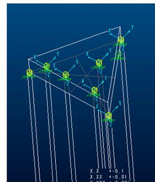
A great deal was learned from the many Mechanica Motion runs with the model. Without the added cables, the design would often “lock-up” due to the non-rotation of the tricorners (it is necessary for proper unfolding that they essentially remained fixed in their original axis plane for the unfolding process). If no loads were applied, but with gravity, the tubes would simply fall over and hang upside down from the cables. This is what one would expect in real life.
