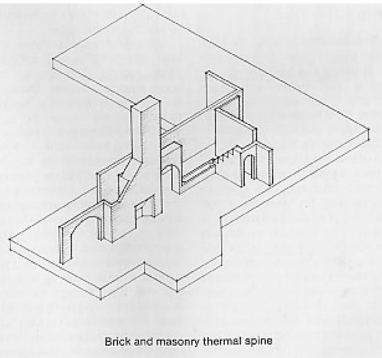
Brick and masonry thermal spine
