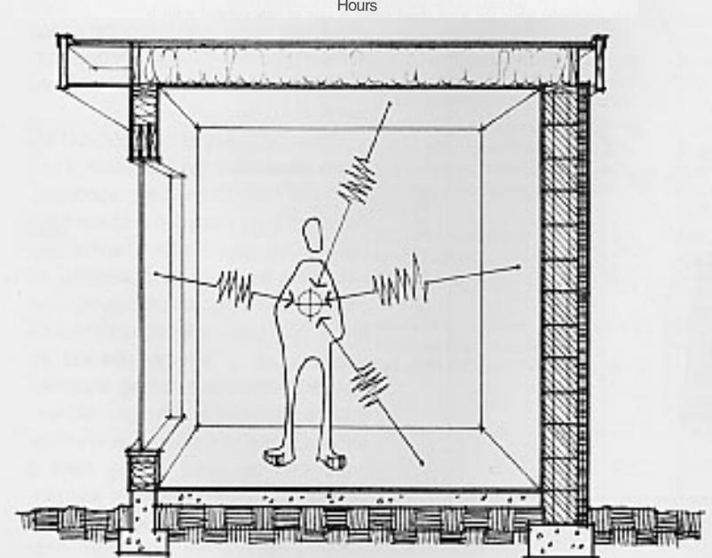
Mean radiant temperature (MRT) is the weighted average of the various radiant surfaces within a space.
